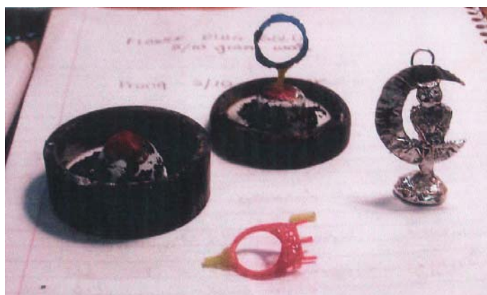
Flask bases, wax models and cast pendant with metal "button" and sprue still attached. (Photograph by Constance Barrow.)
