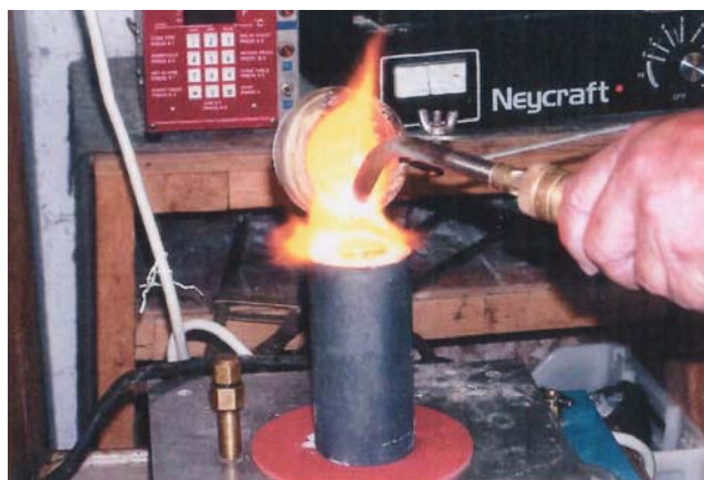
Heating metal in a crucible with a blow torch. (Photograph by Constance Barrow.)
